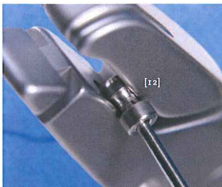
KW protective caps are crimped around proximal KW as shown [12]. This crimping way is only possible with the latest MANOTTE®1.6TB. MANOTTE®1.6TB cuts and bends but also crimps the protective caps we supply.
